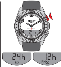
Select mode 12/24 hours - in 12 hour mode, AM appears in the display below the time.
