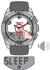
Automatic switch to standby mode after 10 seconds. Beeps every second
